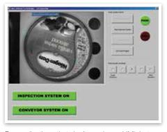
For applications that don't require an HMI, but do require occasional monitoring, the BOA PRO web server provides a run monitor screen that is semi-customizable from the system property page.
