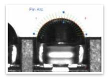
The arc ROI in this image is used to extract points along the surface of a solder ball on a printed circuit board. These points can be used, for example, to calculate the ball radius or find irregularities along the ball surface.
