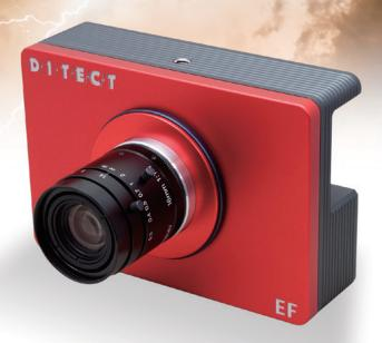
HAS-EF is a high speed camera with 1-inch CMOS sensor and 2,560 × 2,048 effective pixels that can shoot 250 fps at full resolution, 500 fps at full HD, 1,400 fps at VGA, and up to 14,000 fps by limiting the pixel area. Perfect for multiple high speed camera imaging, with 6 GB embedded memory, in one compact solution.
