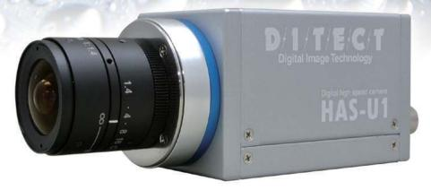
HAS-U1 is a high speed camera with ½-inch CMOS sensor and 1.3M 1280 × 1024 effective pixels that can shoot 200 fps at full resolution, 800 fps at VGA, and up to 4,000 fps by limiting the pixel area. Perfect for multiple high speed camera imaging, with embedded memory, in one compact solution.
