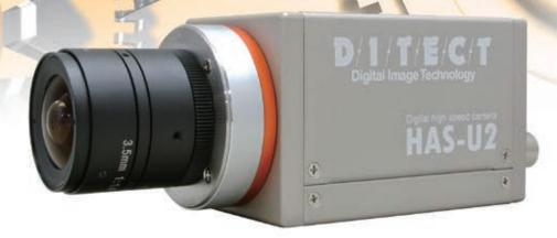
HAS-U2 is a high-speed camera with 1-inch CMOS sensor and 2,592 × 2,048 effective pixels that can shoot 100 fps at full resolution, 1,000 fps at VGA, and up to 7,500 fps by limiting the pixel area.
