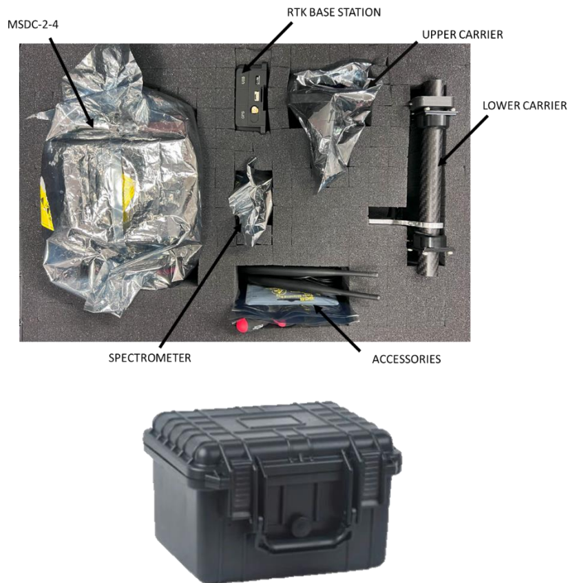
Figure 4. MSDC system package contents.
