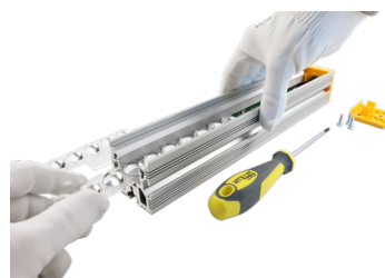
Slide out the window and all lenses
